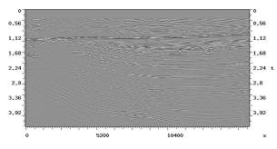
Figure 1: A north-south inline section of the baseline image produced by Chevron (vertical axis two-way travel time in seconds, horizontal axis inline meters).
