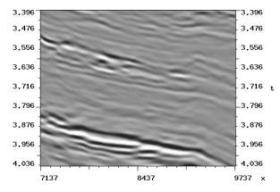
Figure 2: Monitor and baseline image-difference obtained from the 3D time-migration images provided by Chevron and corresponding to the inline section of Figure 1. Productioninduced changes stand out at approximately 3.5 s (wet Illinoisan sands) and 4 s two-way travel times—stacked Neb 1, 2, and 3 reservoirs—compare with Hudson et al. (2005).
